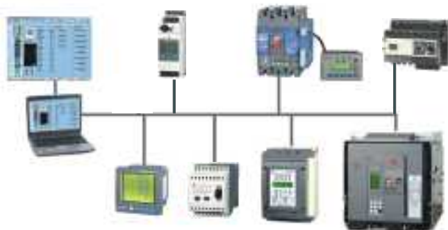
● Ri year-PowerNet配电监控系统
